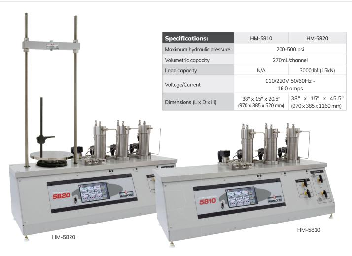
Humboldt's new automated pressure controllers are designed to handle saturation, consolidation and permeation of a triaxial test samples, as well as perform a shear function when using the HM-5020 and its integral Load Frame. Both machines provide a simple and compact setup for doing tests without the need for seperate distribution panels, which simplifies the tubing and and control cable setup.
